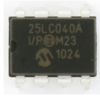
Figure 1.4: EEPROM in PDIP Package
